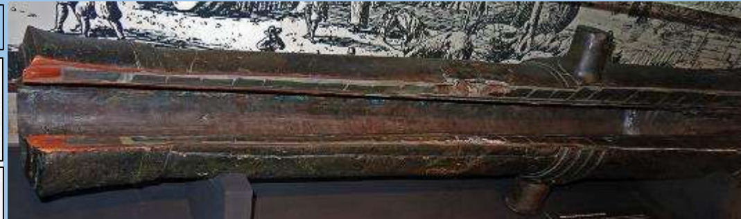
The Composite Drake from the Batavia now sectioned to show sectional construction. Here the main iron tube consists of banded staves indicative of an earlier design than the Fort Nelson example which has a longitudinal tube.
